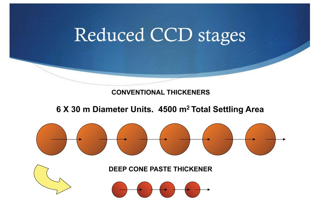
4 x 12 m Diameter Units. 450 m<sup>2</sup> Total Settling Area
