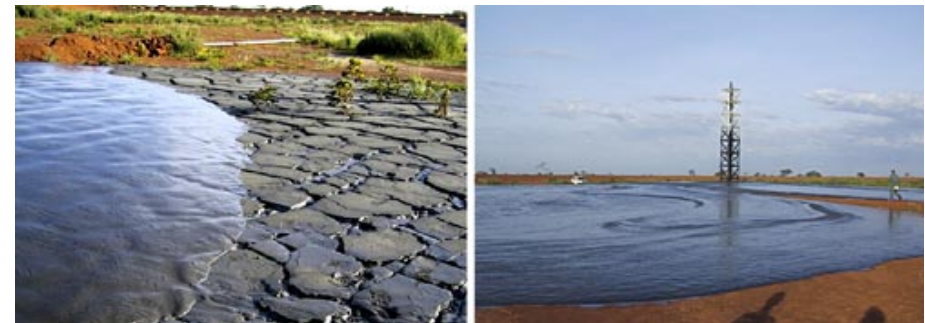
Fresh paste depositing over a desiccated layer (left) and one of the risers at the Bulyanhulu Mine (Barrick), Tanzania (Courtesy Golder Associates)
