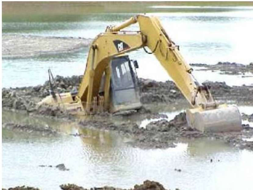
CONVENTIONAL TAILINGS STRENGTH AFTER ???? MONTHS
