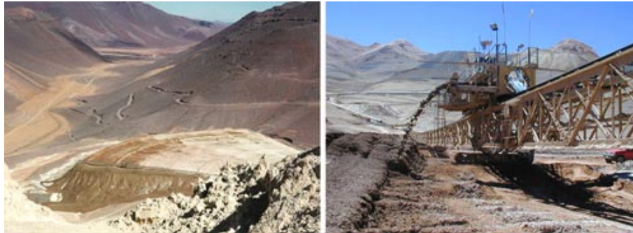
Dry stacking-La Coipa Mine (Anglo American, Chile)
