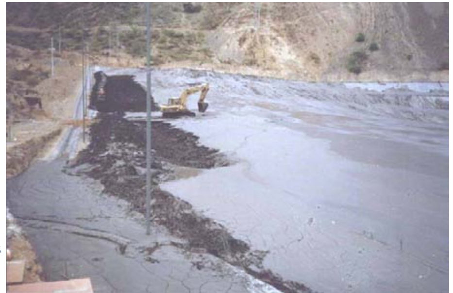
COBRIZA TAILINGS STRENGTH AFTER 4 MONTHS
